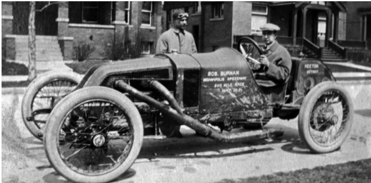
This photo of the sloped grill race car shows Bob Burman at the wheel of the Keeton. Note the open sides reveals the big Wisconsin Motor powerplant. One can only imagine the sound with that massive header hanging off the side!
