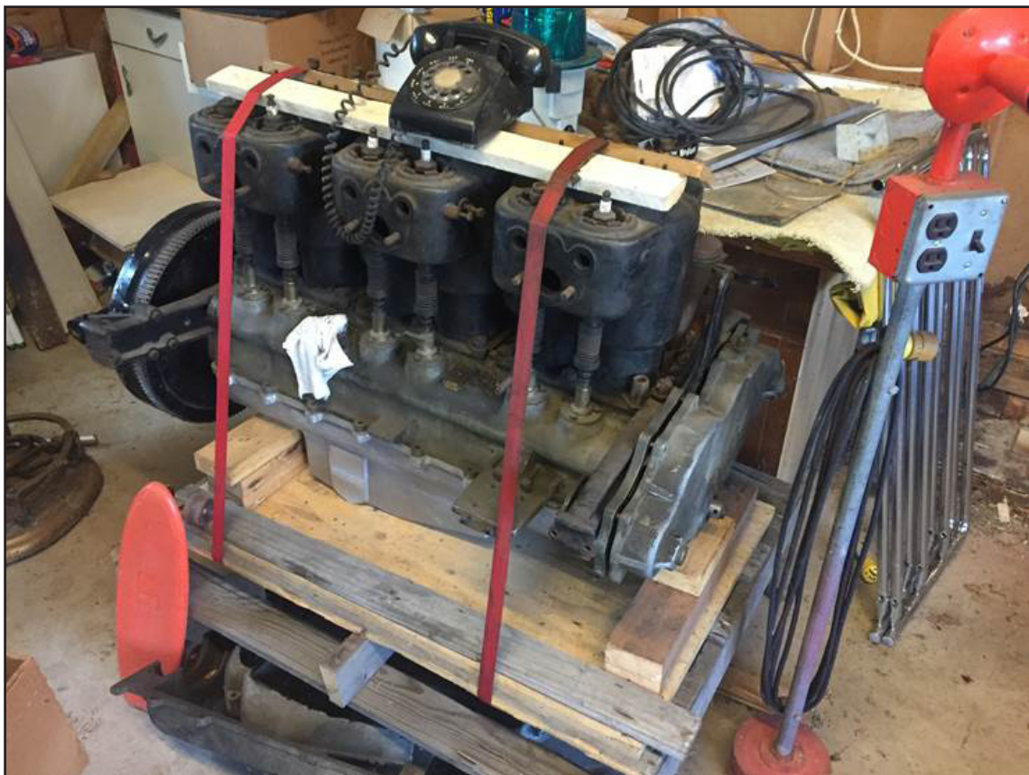
As seen here, the Pierce T-Head has a strong resemblance to the Stutz Wisconsin engine.
