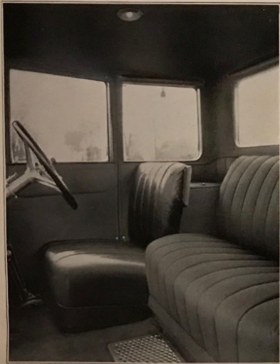
THE interior of the Stutz custom built coupe is very roomy and comfortable and is quite complete in its luxurious appointments. The driver's seat, which is finished in blue Spanish leather, is forward of the main seat for two which is finished in gray, the dominating color scheme of the interior.
