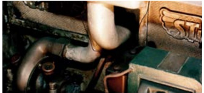
Hot Air Tube Assembly Attaches to exhaust manifold, ducts hot air to carb
