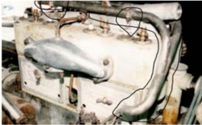
Ignition Wire Conduit & Support Brackets
