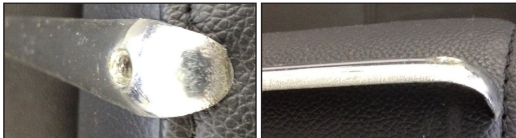
Two views showing the bullet ends that could be reproduced with the new brass moldings.
