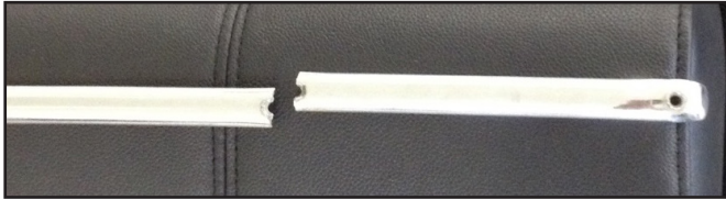
Cracked pot metal molding
