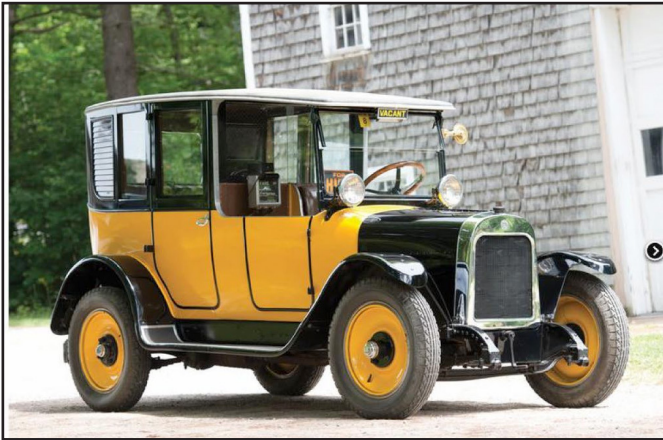
1923 Yellow Cab Model A-2 178.9 cu in. Continental L Chassis No. 12759 head inline four cylinder engine Engine No. 1757V76171 wheelbase 109 in. 18.23 NACC hp
