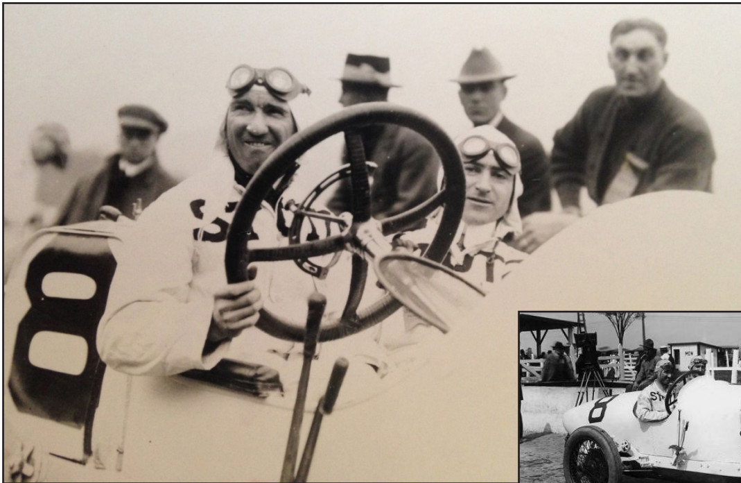
Earl Cooper in #8. Note what appears to be a rock shield that folds down on the steering shaft.
