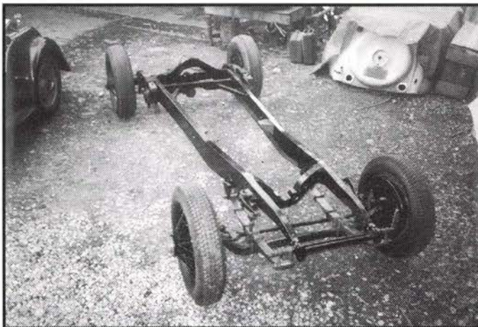
Restored chassis early '91 - new spring length not yet determined.
