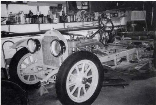
Fitting of fenders to refurbished chassis
