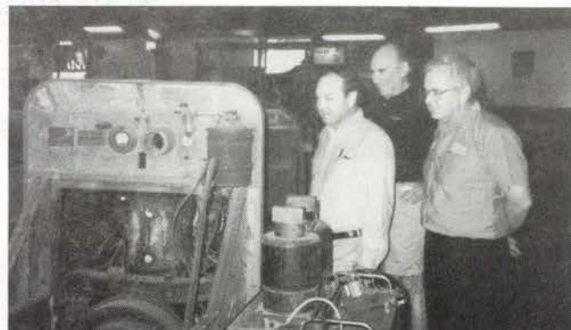
Max Triplett, Ray Katzell and Paul Freehill admire the size and design of SOHC Wisconsin engine. Note heavy cast aluminum cowl and dash.
