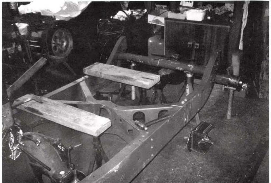
*Chassis cleaned, coated with red oxide*
