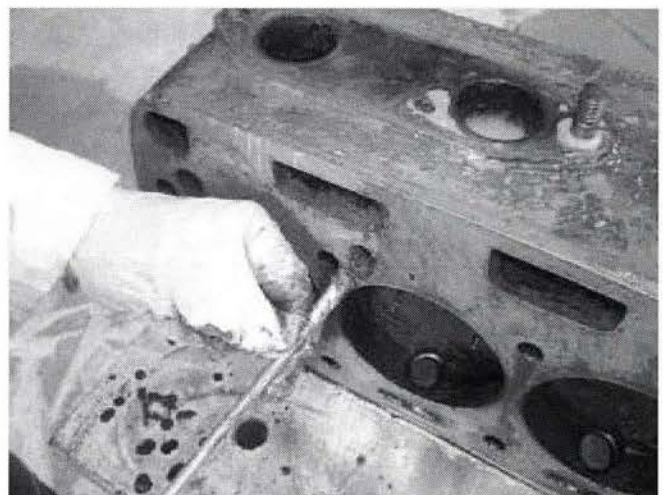
Clearing Rust from the Head
