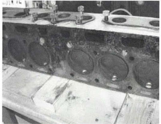
Head Removed for Valve Lapping
