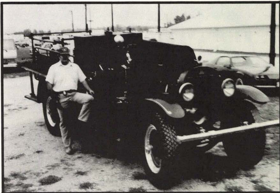
Jeff Henry with Member Jim Dougherty's 1921 Stutz Model "B" #666 600 G.P.M. Pumper at the 1st Grand Stutz at Indianapolis in September 1988. The model "M" Motor #593 has a 5-3/4" bore x 7" stroke. The big 8./liter 4 cyl. T-Head purrs like two Bearcats! Ed.
