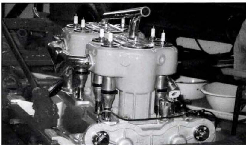
Early assembly. Note the Gemmer steering box (left) which we made, writes Kraft.
