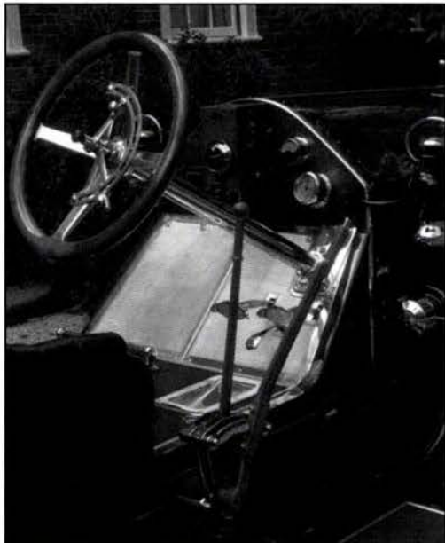
Note fitted aluminum dash plates and footrests for driver and passenger and the rubber mat as mentioned in text.
