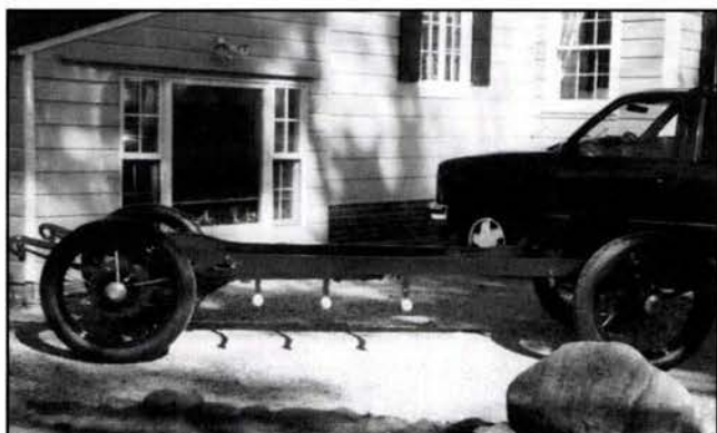
The Bearcat chassis now with dead brakes and wheels. Next comes installing the motor etc.
